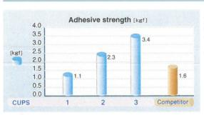
Adhesive strength: Suction a pig heart at -300mgHg and pull up vertically, and measure the force of detachment.
